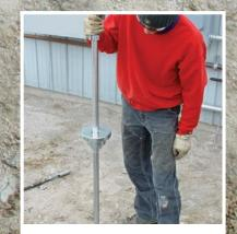
Dynamic cone penetrometer. Part #59000. Evaluate strength and density of soil, in situ.
