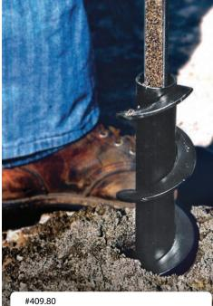
Collect soil, soil gas, or groundwater samples telescopically through AMS hollowstem augers.
