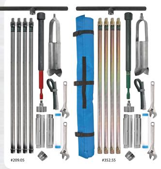
AMS split-core sampling kits provide everything you need to auger to 12' and collect a virtually undisturbed soil core sample into the split-core sampler body or into a liner. The kits utilize 5/8" threaded or signature series connections, and all of the augering and sampling components are made entirely of stainless
