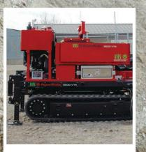
Geotechnical Sampling and testing can also be conducted with AMS PowerProbe<sup>™</sup> and direct push tooling. [Page 93]
