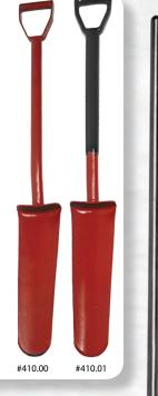
Stainless Steel Spade Shovel Durable stainless steel construction withstands caustic and corrosive materials and is easily decontaminated after use. The blade of the AMS spade shovel has a front-rolled step, a fine cutting edge, and measures 7 3/4" x 11". The overall length of the shovel is 54".
