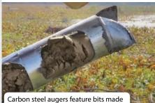
of high-carbon steel with heat-treated tungsten carbide hard-surfaced edges.
