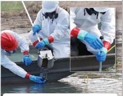
The dredge can be triggered to close using the messenger and rope, or by pushing on the top of the optional handle.
