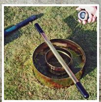
Infiltration rings. Part#400.97. Monitor infiltration rates, and study liquid waste disposal, leaching, and drainage efficiencies.
