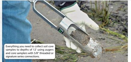
AMS basic sampling kits provide everything you'll need to auger to a target depth as deep as 12' and obtain a relatively undisturbed soil core sample. The kits are used worldwide by soil scientists, agronomists, and construction companies for site investigations.
