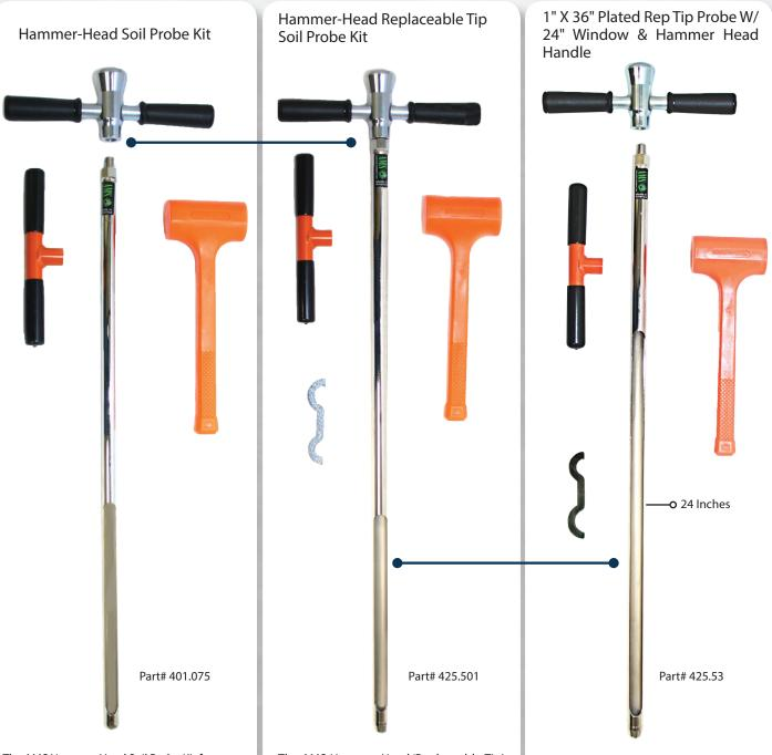
The AMS Hammer-Head Soil Probe Kit features a 16"L hammer-head cross handle which can be hammered on with the (included) impact absorbing dead blow hammer. No need to lug around a heavy slide hammer anymore! A standard 10" cross handle with rubber grips also comes in the kit for regular soil conditions. Probe measures 7/8"-dia. x 33"L and is constructed of nickel plated chrome molybdenum. Hammer head is made of highcarbon, stress-proof steel.
