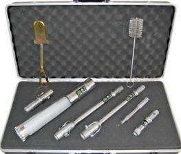
through those dreaded frozen soil conditions. The kit comes with the core barrel auger, two 1ft. hex quick pin extensions, two threaded/hex quick pin adapters, SDS-Max rotary hammer drill adapter, Idaho spoon cleanout tool, SST cleaning brush & one hard side carrying case with foam lining. The kit is designed to work with an SDS-Max rotary hammer drill, but may be adapted to a Tanaka TIA-350PFS Gas Drill for added portability.
