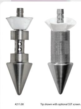
Dedicated gas vapor tips are installed as long-term sampling points or left in the ground as expendable points. They are used for detecting hydrocarbon spills, underground storage tank and pipe leakages, landfill contamination, and hazardous waste sites. Soil gas monitoring with the AMS dedicated gas vapor tip is easily accomplished using a slide hammer or electric rotary hammer drill with GVP extensions and an extension drive adapter. GVP kits are available. See pages 51-53.
