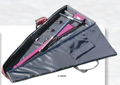
\* The TDR 300 Turf Soil Moisture Meter Kit includes the TDR 300 meter, an AMS Turf Probe, two 4.8" SST Rods, two 8.0" SST Rods, and a soft-sided carrying case.
