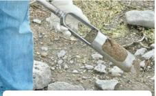
Stainless steel (SST) kits have SST extensions and augers made with SST bails, cylinders, and bits.
