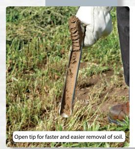
Open-end probes collect shallow soil samples (15" in length). They are primarily used for agricultural applications. The probe body is made from nickel-plated chromoly. The 15" slot in the probe is cut to the end of the probe body to facilitate emptying of the sample. It includes a 10" handle.
